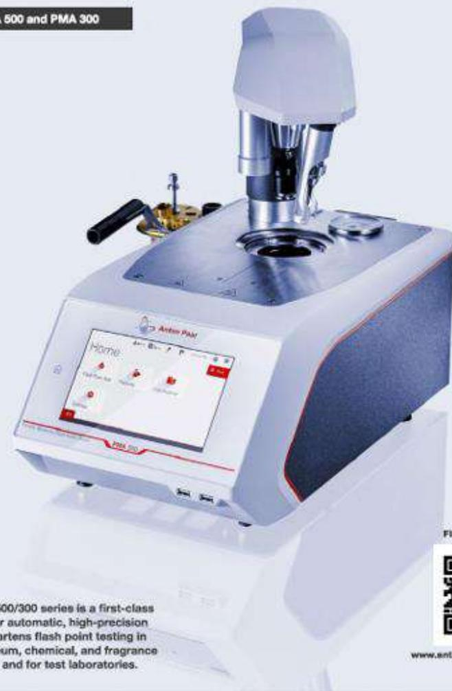
The PMA 500/300 series is a first-class solution for automatic, high-precision Pensky-Martens flash point testing in the petroleum, chemical, and fragrance industries, and for test laboratories.
