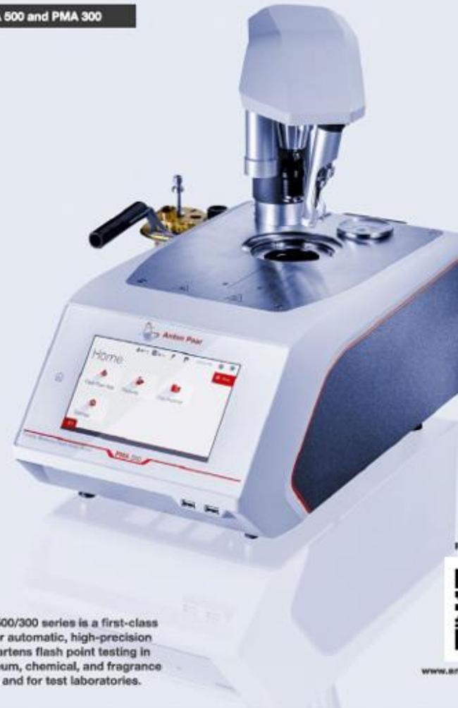
The PMA 500/300 series is a first-class solution for automatic, high-precision Pensky-Martens flash point testing in the petroleum, chemical, and fragrance industries, and for test laboratories.
