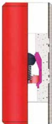
COLLAR DE FLOTACION CON SOLDADURA A TOPE CON VÁLVULA DOBLE
